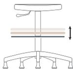
height adjustment by gas lift. Allows a 13 cm excursion for the seat with a 5-star base on castors, 26 cm for the stool with feet.
