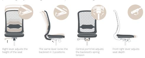
synchronised self-calibrating with 3-position adjustment (oscillation angles: position 0: backrest 0.4° seat 1.5°; position 1: backrest 7.9° seat 0.76°; position 2: backrest 16.9° seat 3.3°) and anti-shock release system. This mechanism allows the backrest to adapt automatically to the user's weight without requiring any operation. The backrest tilt resistance is directly proportional to the weight exerted on the seat.
