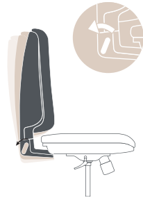
Lever on the backrest locks and unlocks the backrest
