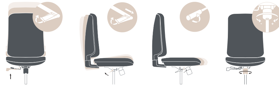
Front right lever adjusts the seat depth
