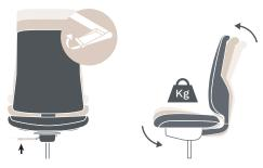
Right lever adjusts the height of the seat
