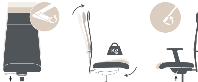
Lever on the right, to adjust the seat height
