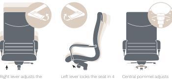
Right lever adjusts the height of the seat
