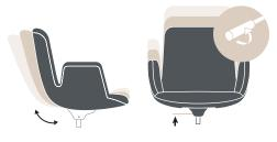
Right hand lever adjusts the height of the seat
