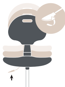
Right lever adjusts the height of the seat
